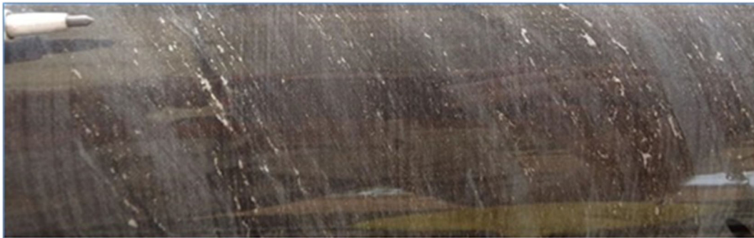
Figure 7.7: Photograph of abundant, foliation controlled, coarse grained arsenopyrite (From KNDD0001: 176.4m (2.23 g/t Au))
