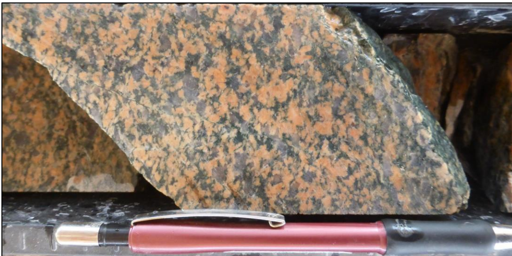
Figure 7.13: Distal alteration: hematite-chlorite pervasive alteration
