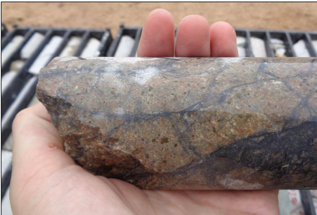
Figure 7.15: Strong silica-sericite alteration - high grade mineralisation
