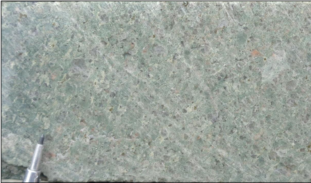
Figure 7.14: Proximal intense sericite and fine grained disseminated pyrite alteration
